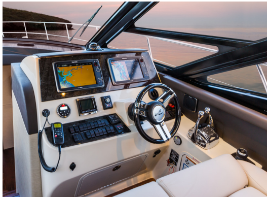
This advanced helm deserves to be called "mission control" thanks in part to its standard Zeus® propulsion joystick and Raymarine e125 widescreen GPS/chartplotter/radar unit.
