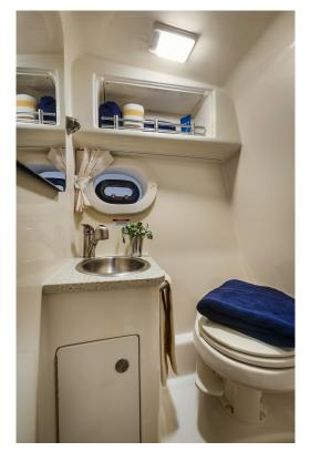
The full fiberglass stand up head includes a convenient portable head or optional VacuFlush® head with holding tank.
